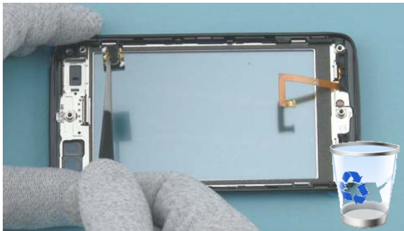
44) Remove the earpiece with the tweezers. The earpiece adhesive cannot be reused.
