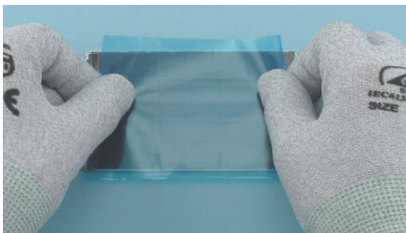
42) Remember to protect the LCD display with a protective film.
