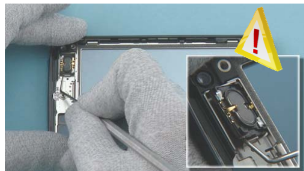
43) Use the dental tool to release the earpiece.
