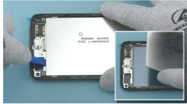
41) Use the SS-93 to lift up the LCD display and then remove it.
