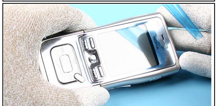
56. Check the windows for cleanness.
