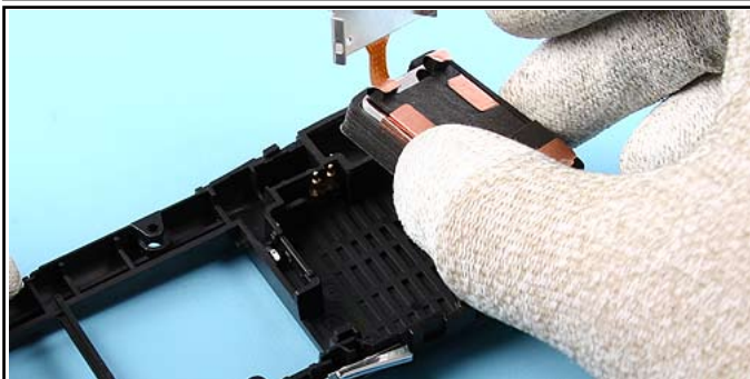
51. Lift out the HDD ASSEMBLY. Never remove it by pulling at the flex foil.
