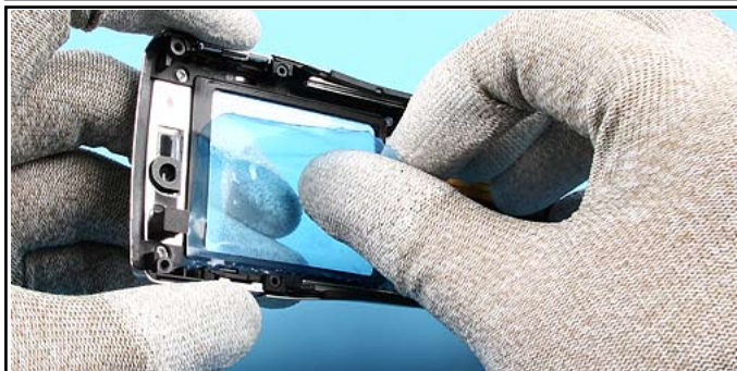
11. Protect the inner side window with a plastic film.
