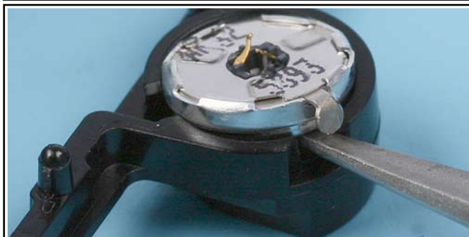
27. Lift up and remove the EARPIECE with tweezers carefully.
