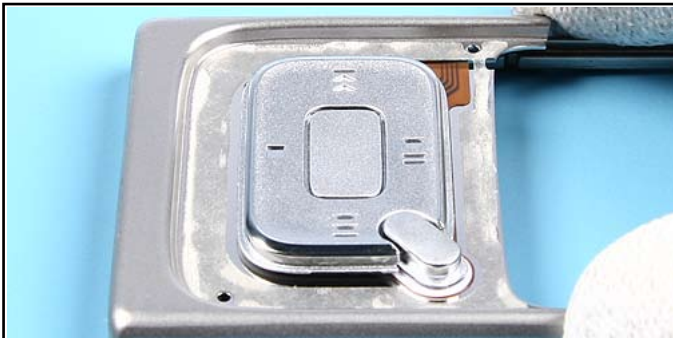
21. Remove the adhesive residue.
