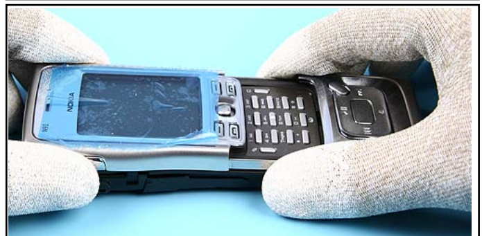
52. Check the functionality of the RAIL SPRING. The SLIDE ASSEMBLY must be stop safely at the end position.
