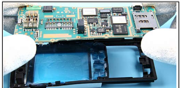
20. Use the A-COVER as support when replacing the CAMERA MODULE.
