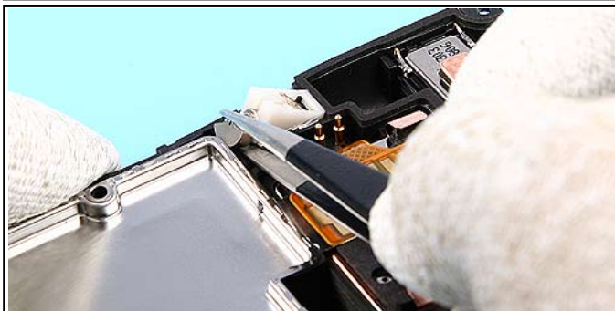
35. Remove the VIBRA ASSY.
