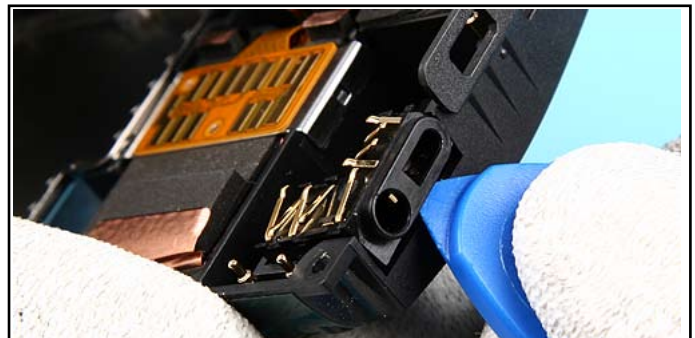
38. Lift the 3,5 AUDIO JACK and remove it.
