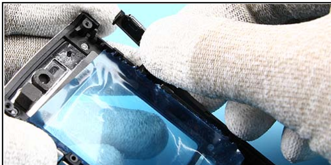
13. Pull out the VOLUME KEY HARDTOP...
