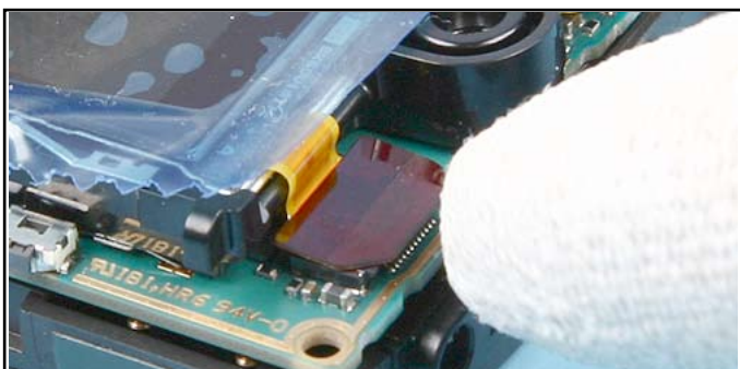
33. Note the correct position of the flex connector before continuing.
