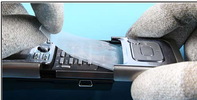
51. Place a piece of plastic film while assembling the SLIDE ASSEMBLY. Remove the plastic film carefully while shifting the parts together .
