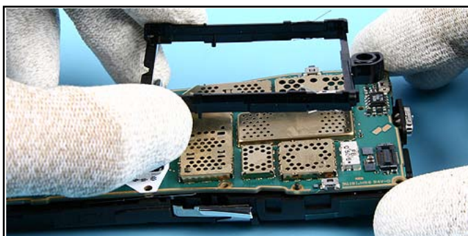
25. Remove the DISPLAY FRAME ASSEMBLY.
