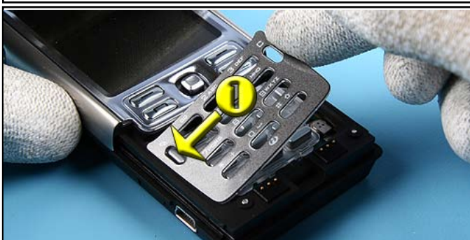
47. Place the BEZEL COVER at the shown side first.
