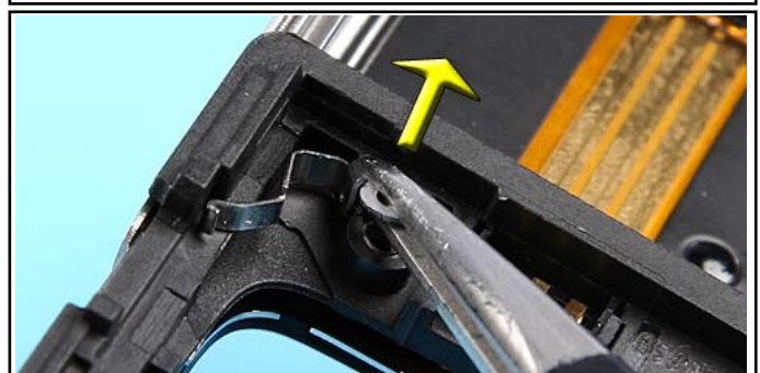
16. Pull it out carefully with tweezers.
