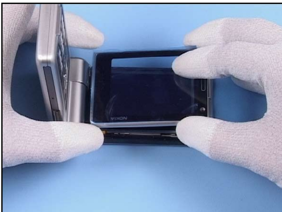
29. Place the B-Cover , beginning from the hinge side. Push it down evenly at the corners.
