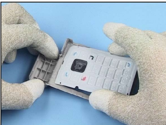
23. Insert the Keymat . Do not touch the adhesive surface.
