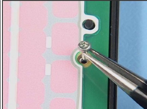
14. Insert the two short screws.
