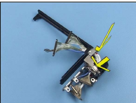
11. Red marks on the Coax Cables must be visible.
