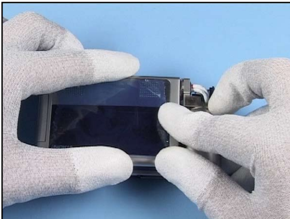
39. Push down at the hinge side to click the clips into their places.
