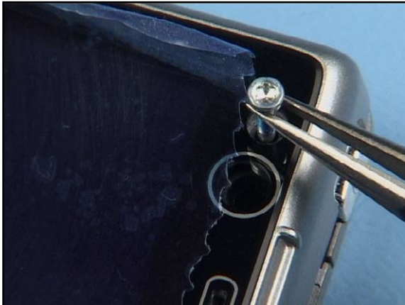
31. Insert new screws.
