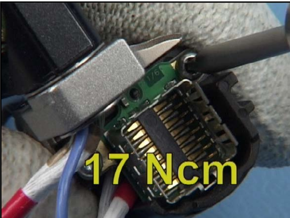
9. Tighten the screws with the correct torque.
