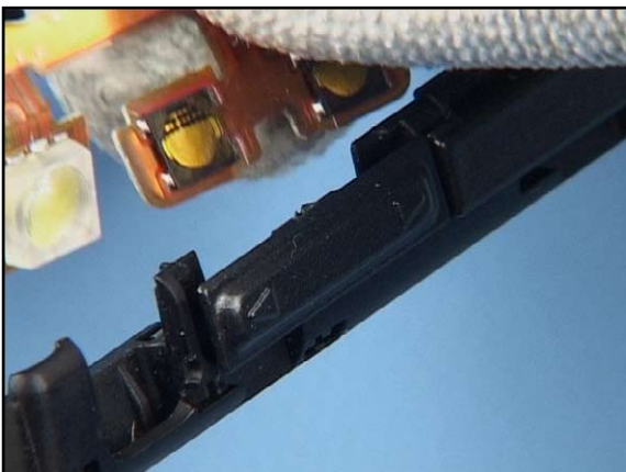
23. Carefully pull out the Bottom Frame Flex Assy .
