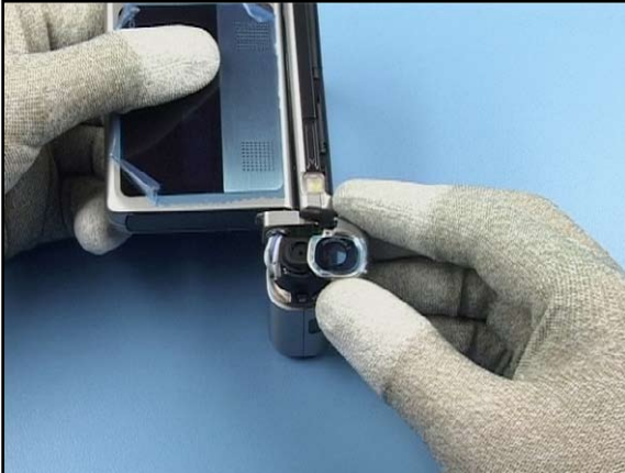
43. Turn the assembly into position shown and place the Hinge Cover B first.
