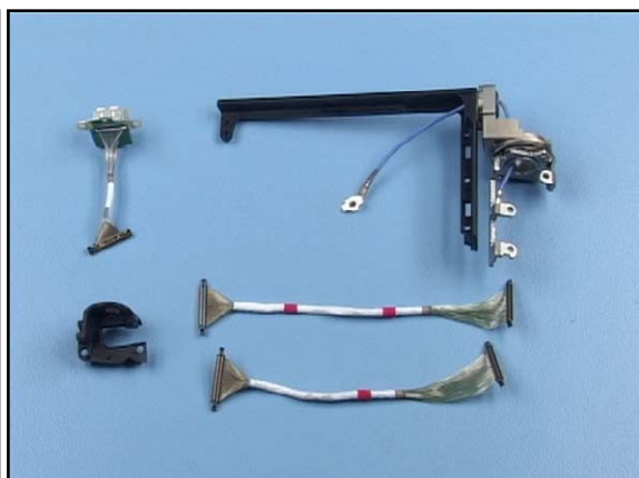
12. Now the disassembly of the Hinge assy is completed.
