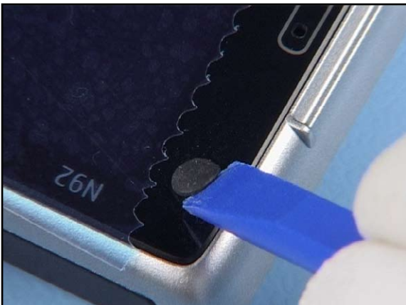
15. Prevent scratching the window while removing the Bumper Plugs .
