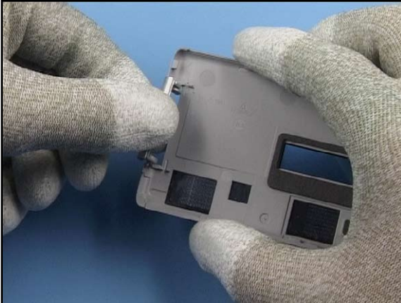
37. Assemble the Memory Card Door not already done before going on.
