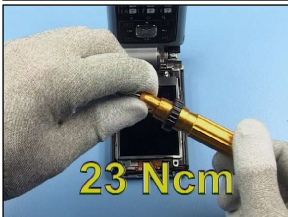
23. Set the correct torque.
