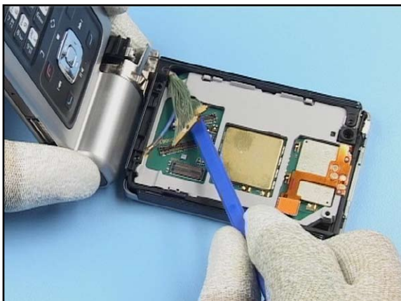
30. Remove them completely with the SS-93.
