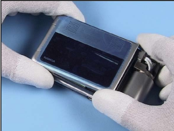
13. Use the SS-45 camera removal tool to release the Camera Module 2Mpix as shown.
