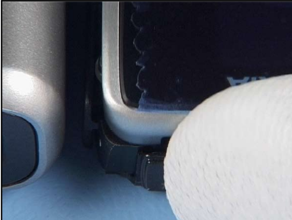
19. Lift up the B-Cover Assy carefully and release all clips.
