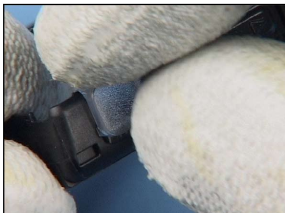
6. Insert the Flash Lens .
