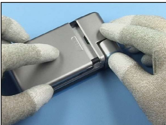
47. Complete the Unit with the Battery Cover .
