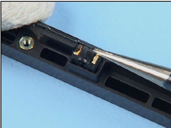
27. Pull out the Microphone.
