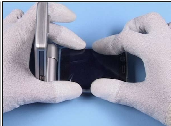
30. Now smooth it down evenly to click the side clips into their places.
