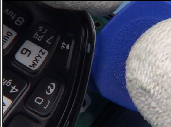
8. Release the glued Keymat , beginning at the edge with the SRT-6, mind the dome sheet.
