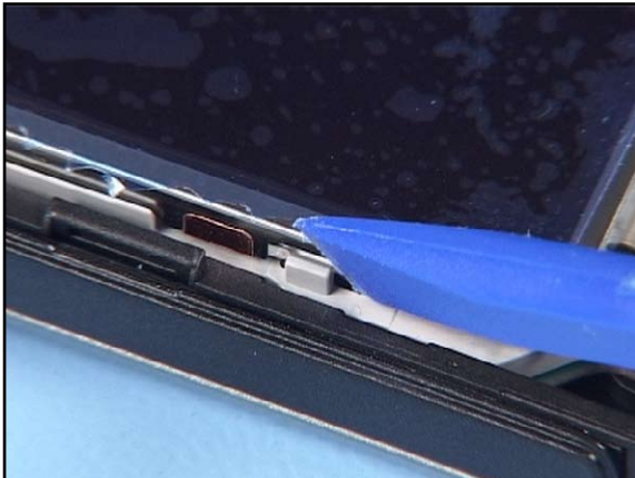
25. Carefully release and remove the clips of the Display Frame Assy.
