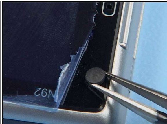
34. Place the Bumper Plug . Do not scratch the window.
