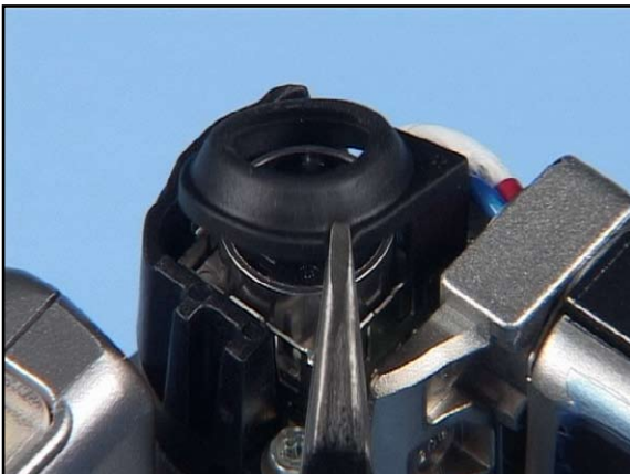
9. Remove the Camera Window Elastomer .
