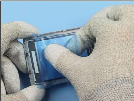
21. Cover the inner side window with a plastic film.
