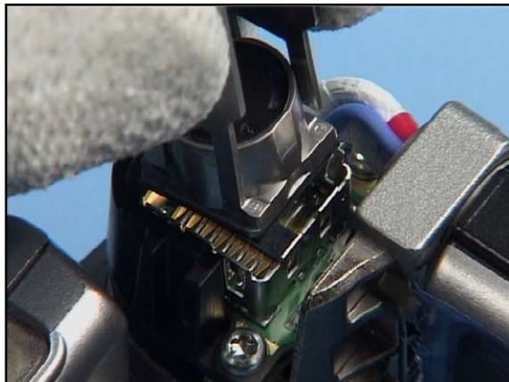
10. Use the SS-45 camera removal tool to release the Camera Module 2Mpix as shown.
