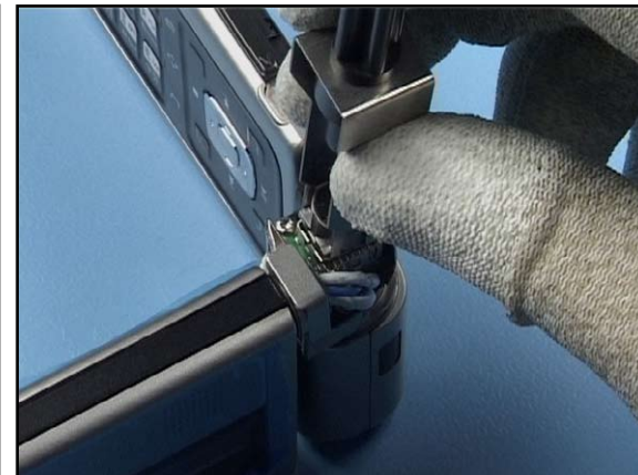
40. Use the SS-45 camera removal tool to assemble the Camera Module 2Mpix as shown.
