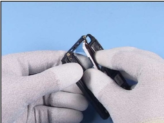
39. Remove the 2nd Display Module.
