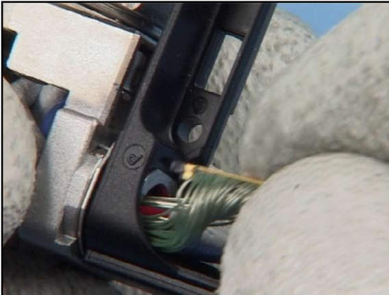
7. Carefully twist the connector of the Coax Cable . Now pull the cable while slotting the connectors through the recess of the Hinge Module Assy .
