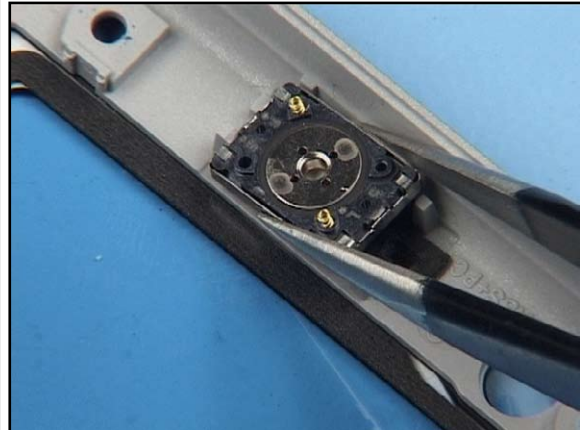
26. Insert the Earpiece . Always use a new Gasket.
