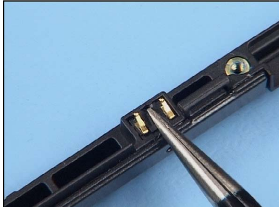
2. Insert the Microphone into its recess.
