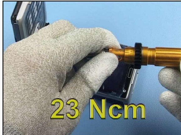
32. Set the correct torque.
