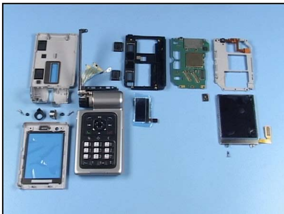
42. The disassembly procedure of the upper block is now complete.
