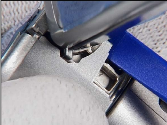
7. Carefully release the clip of the Hinge Cover B ...
