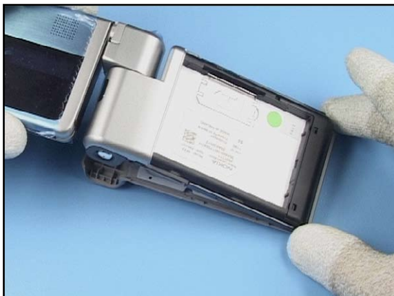
24. Turn the unit and join the parts, beginning from the bottom. Click all snaps into their places.
