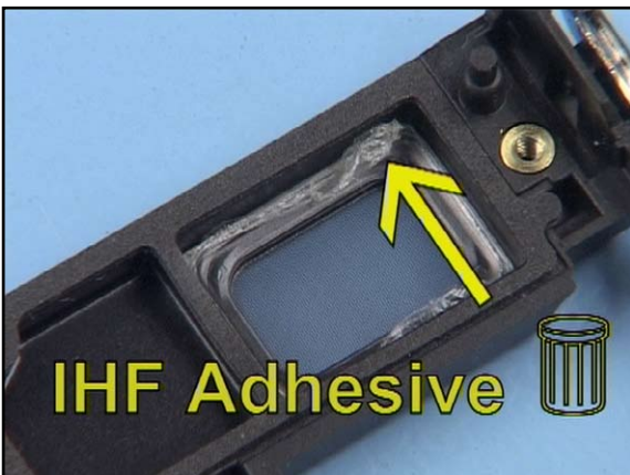
41. Always use a new IHF Adhesive when reassemble.
