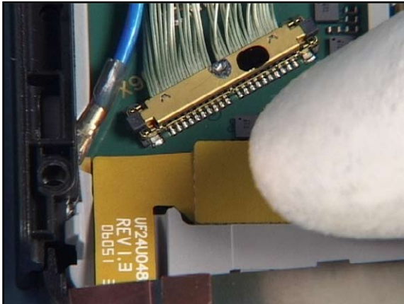
19. Close the display connector.
