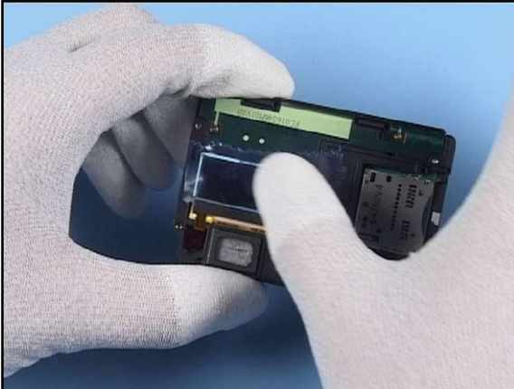
13. Cover the display with a protective film.
