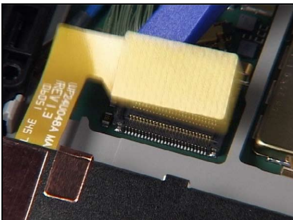
27. Open the connector with the SS-93.
