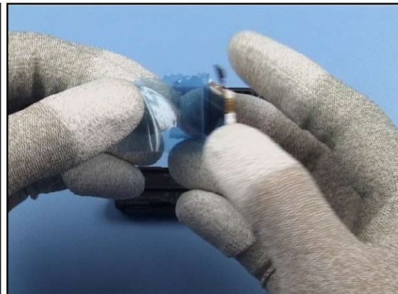
4. Remove the plastic film from the 2nd Display Module.
