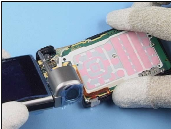
14. Now the parts can be separated.
