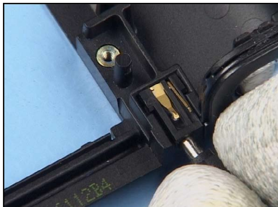
4. Insert the DC Jack into its compartment.
