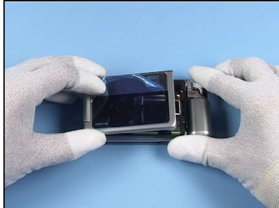
38. Place the A-Cover over the assembly, shift it carefully into hinge direction.
