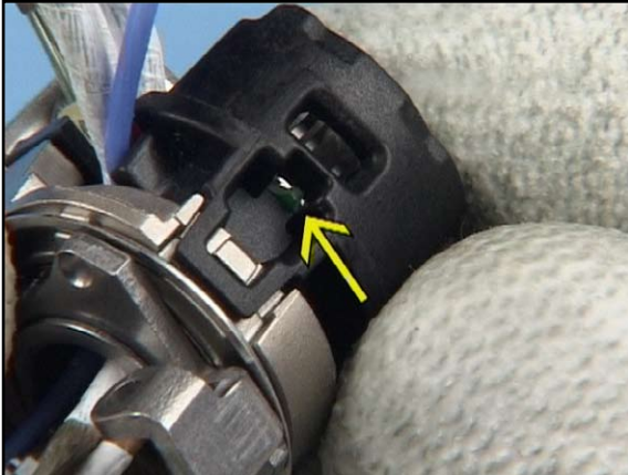
7. Note the correct positioning of the alignment tab.
