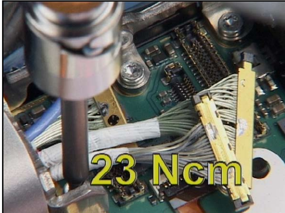
20. Tighten these screws with the correct torque.
