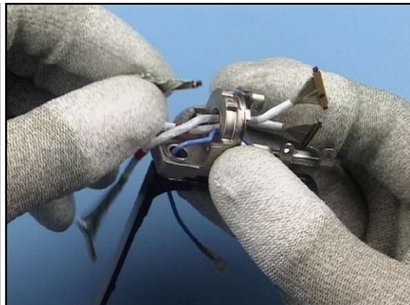
10. Carefully twist the connector of the Coax Cable . Now pull the cable while slotting the connectors through the second recess of the Hinge Module Assy .
