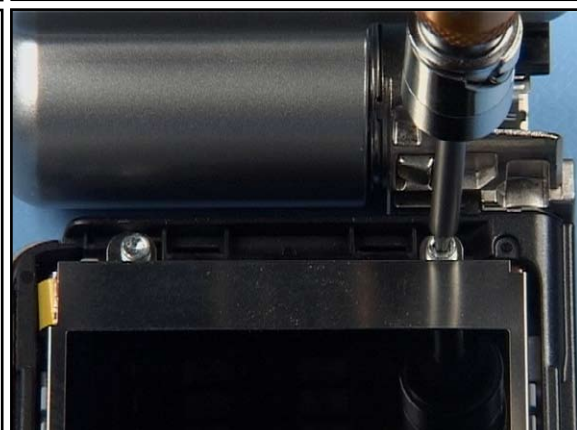
24. Tighten both screws.
