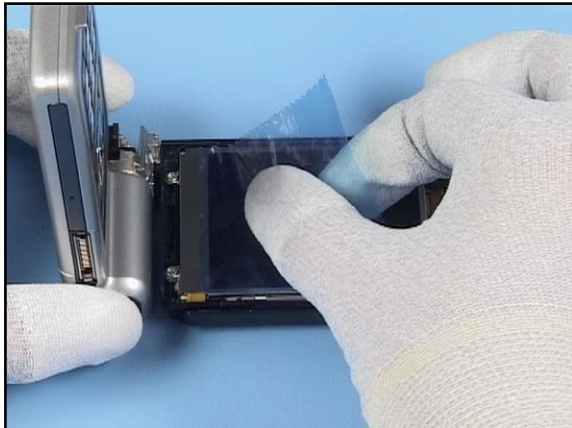
22. Cover the display with a protective film, too.
