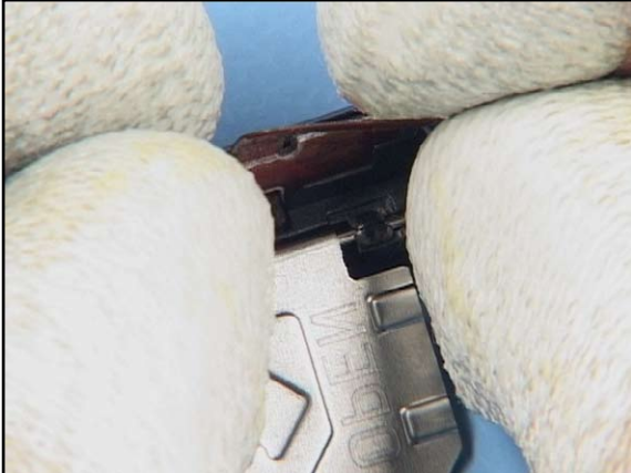
7. Now insert the Bottom Frame Flex Assy .
