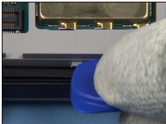
34. Release the snap as shown.
