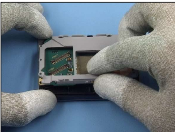
35. Now the Spacer Frame Assy can be removed.
