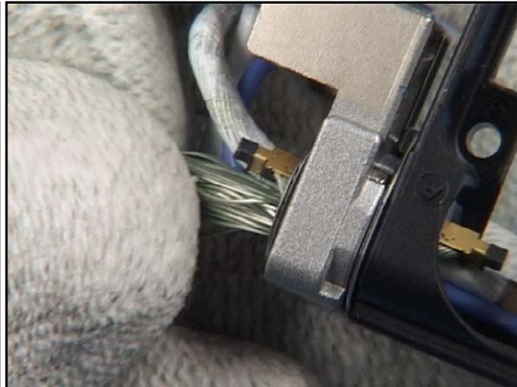
8. Note that the cables are not squeezed during this procedure.
