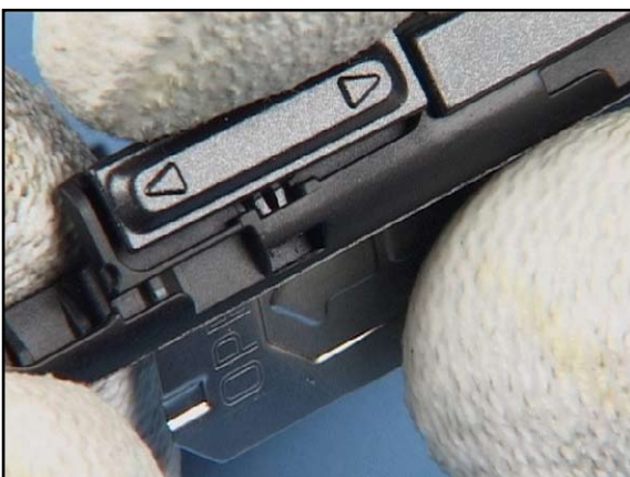
5. Place the Volume Button into the Bottom Frame Assy .
