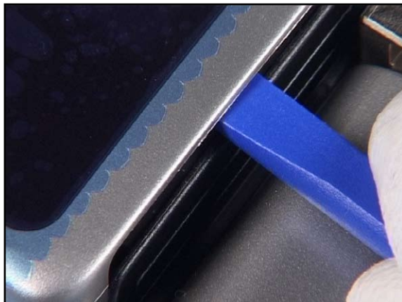
12. Release both clips on the hinge side too. Note that these clips are very delicate.
