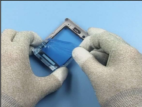
25. Peel up the protective film first.
