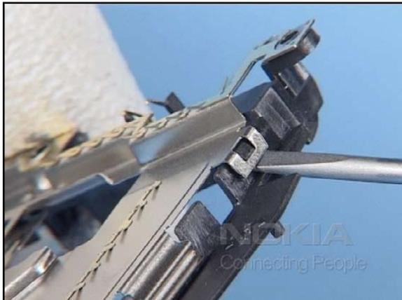
28. Lever up the first metal latch of the BB SHIELD
