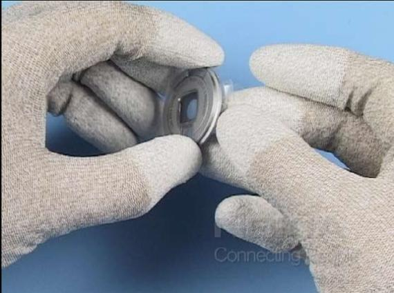
7. Remove the protection film from the CAMERA PROTECTIVE SHUTTER.
