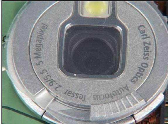
38. Ensure that the protection film is still fitted, otherwise protect it with a plastic film.
