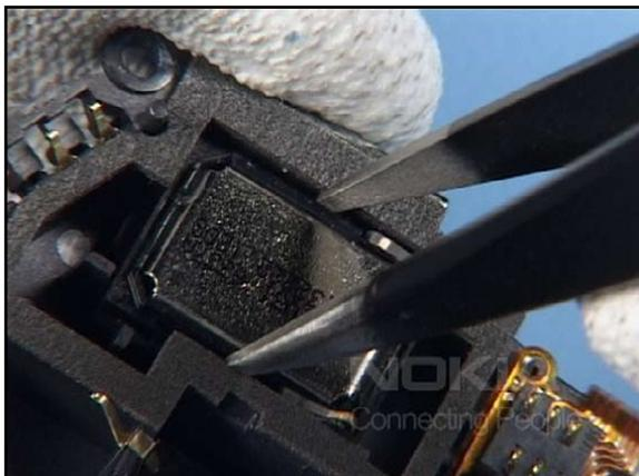
12. Mind the correct positioning before placing the speakers into the CHASSIS.
