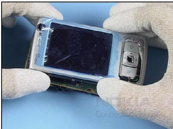
30. Bring the slider into position shown while placing it over the lower part.
