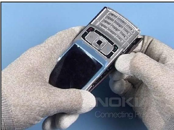
5. Bend open the BACK COVER ASSEMBLY carefully.
