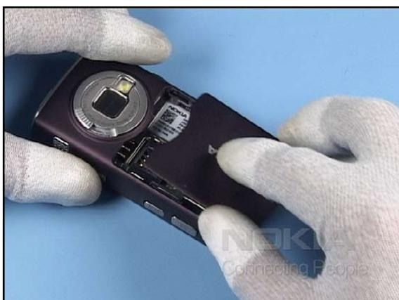
48. Complete the assembly with the BATTERY COVER.
