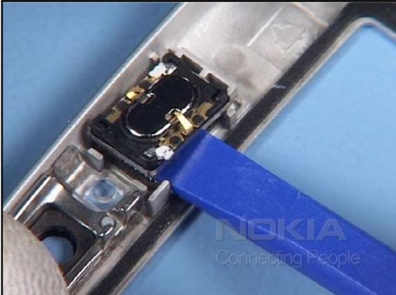
19. Gently release the adhesive of the EARPIECE. The gasket will be destroyed while removal.
