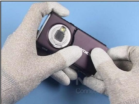
3. Unlock and remove the BATTERY COVER.
