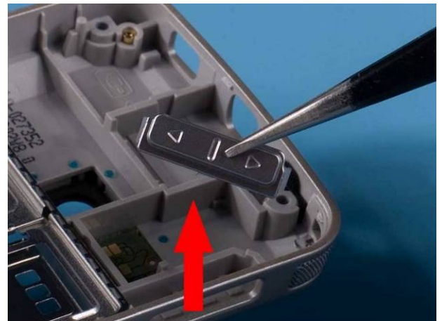
40) Use finger to push on VOLUME KEY and remove it with tweezers.
