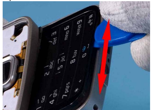
10) Use SRT6 to release snaps of T9 KEYMAT ASSEMBLY.
