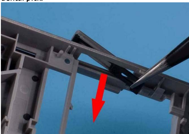
35) Open MICRO SD CARD DOOR and remove with tweezers.
