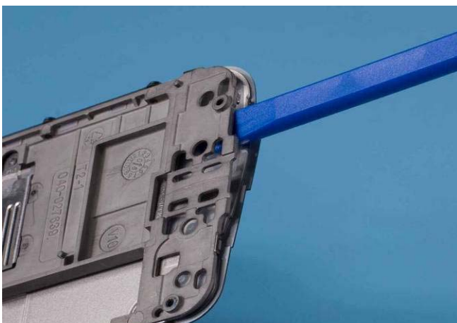
29) Use SS-93 tool to release MEDIA KEYMAT ASSY.
