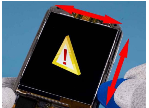
16) Insert SRT6 and slide along edges to lift up DISPLAY ASSEMBLY . Be careful not to damage the LCD .
