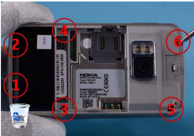
3) Remove 6 screws using a TORX6 screwdriver.
