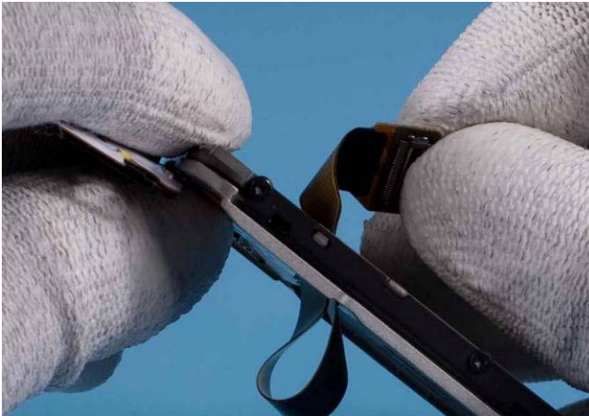
19) Guide connector through SLIDE ASSEMBLY .
