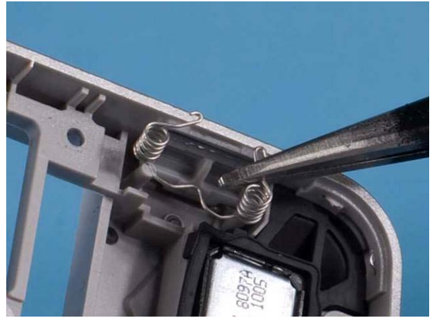
44) Use tweezers to lift up SHUTTER KEY SPRING .
