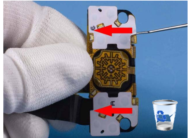
26) Use dental pick to peel off S60 MAIN DOMESHEET.
