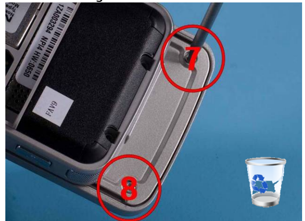
4) Remove 2 screws using a TORX6 screwdriver.
