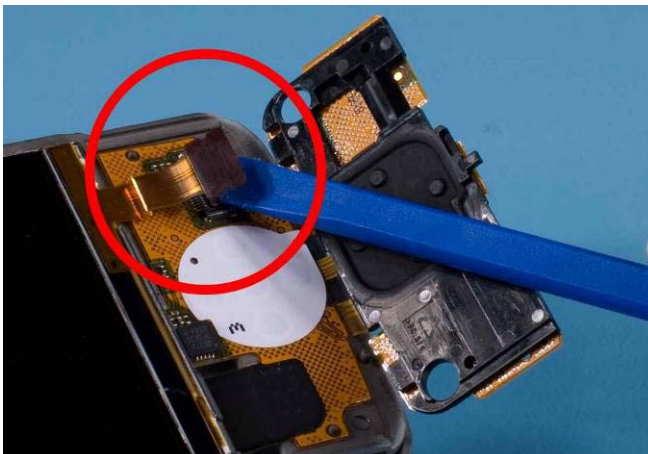
15) Release LCD connector using SS-93 tool.
