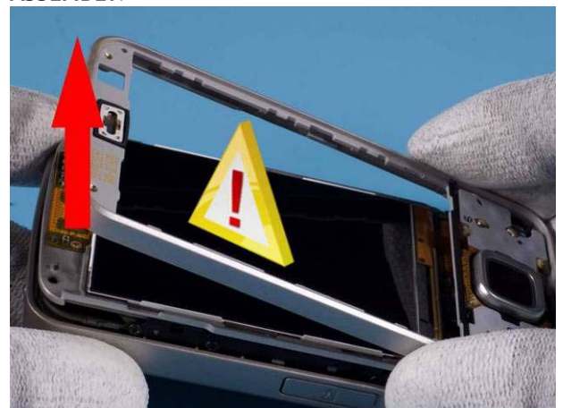
12) Carefully lift up A-COVER to remove it.
