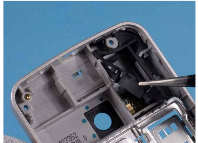
38) Use tweezers to remove SPEAKER BOOT UPPER .
