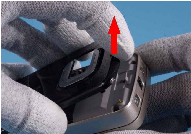
1) Push down on latch and pull up the BATTERY COVER .
