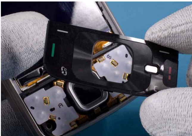
9) Separate MENU KEYMAT ASSEMBLY from A-COVER.
