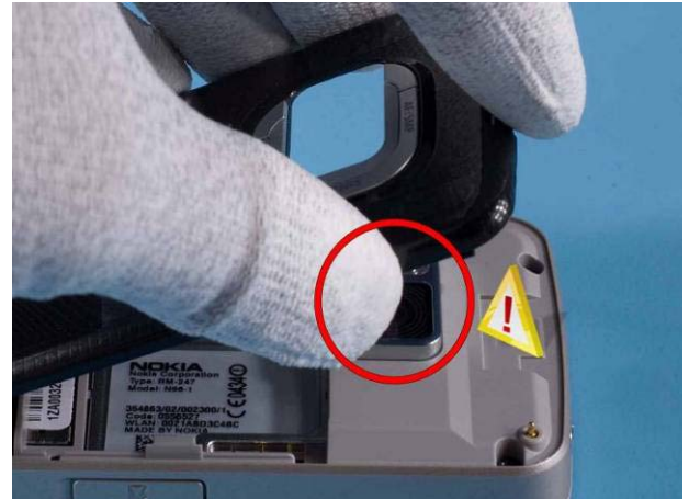
2) Lift up BATTERY COVER . Be careful with the camera housing .
