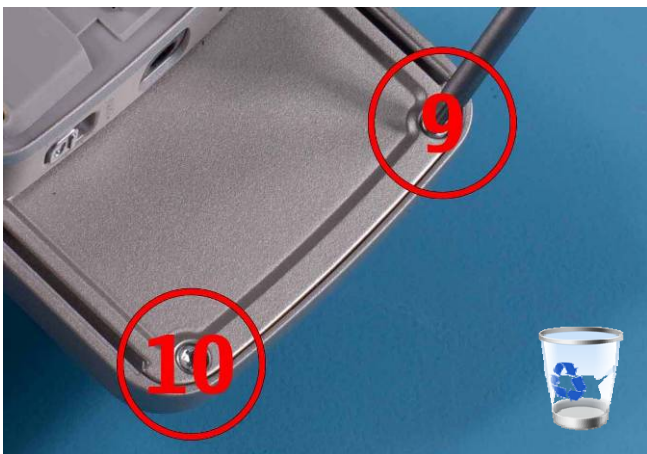
5) Remove the 2 remaining screws.
