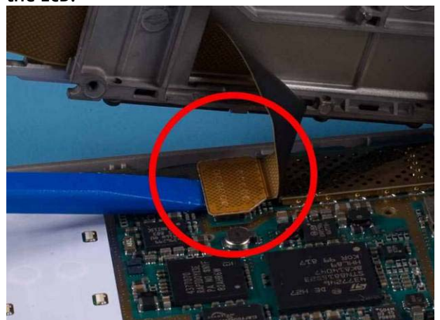
18) Use SS-93 tool to release the connector.
