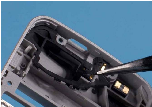
47) Use tweezers to remove SPEAKER BOOT LOWER .
