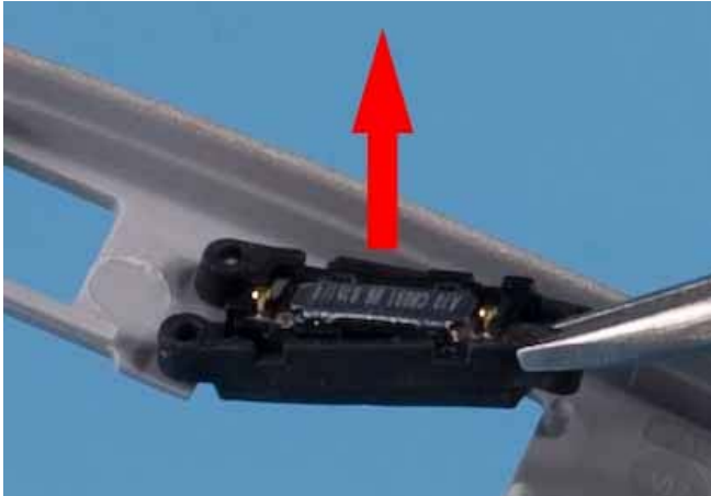
13) Use tweezers to remove the EARPIECE BOOT with EARPIECE .
