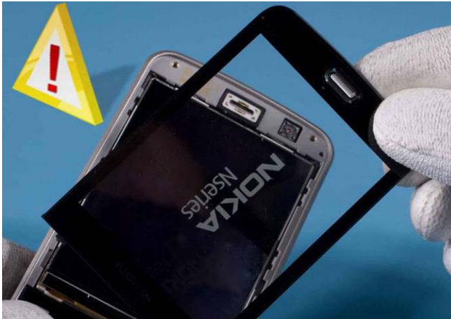
7) Carefully lift up the WINDOW ASSY.
