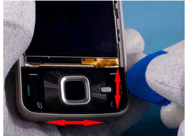
8) Insert SRT6 and slide along edges to release clips.
