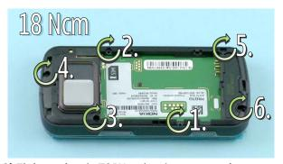
3) Tighten the six TORX + size 4 screws to the torque of 18 Ncm in the order shown.
