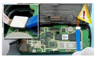
14) Then open carefully the Q-ROCKER FPC ASSEMBLY CONNECTOR with the SS-93.
