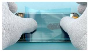
34) Remember to protect the LCD with protective film.
