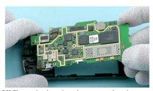
22) The engine board can be separated as shown.
