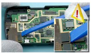
16) Use the SS-93 to open the connector of the AUDIO FPC ASSEMBLY. Be careful not to damage the connector - or components nearby.
