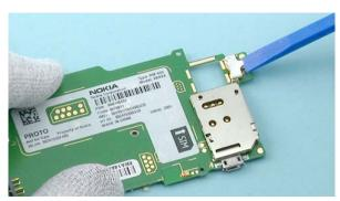
26) Release the HEAT SINK ASSEMBLY with the SS-93 and then remove the assembly.
