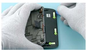
31) Detach the A-cover assembly with the SRT-6 as shown.
