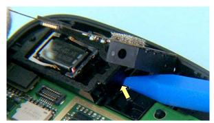
18) Then release the IHF HOLDER ASSEMBLY with the SS-93.
