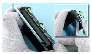
10) Slide the SRT-6 along the cover to release all the clips.
