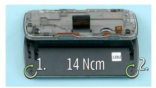
1) Tighten the two Phillips size 00 screws to the torque of 14 Ncm in the order shown.
