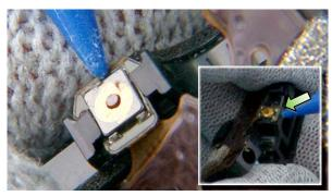
20) Use the SS-93, to separate the AUDIO ASSEMBLY and the IHF HOLDER ASSEMBLY.
