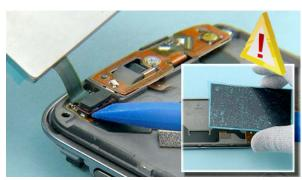
37) Disconnect the LCD connector with the SS-93. Then remove the LCD.
