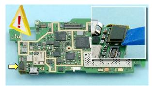
24) Next, open the connector of the BEZEL FPC ASSEMBLY with the SS-93.
