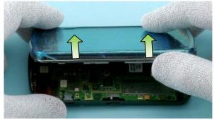
12) Carefully lift up the upper part to gain access to the TILT FPC ASSEMBLY connector.
