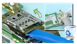
25) Turn the ENGINE BOARD over and use the SS-93 to release the BEZEL FPC. Then remove it. Do not use the BEZEL FPC again.
