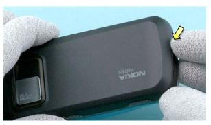
4) Press release button and remove the BATTERY COVER.
