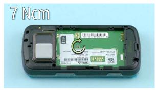
2) Tighten the TORX + size 4 screw to the torque of 7 Ncm.
