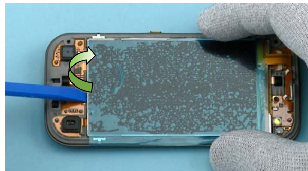
34) Use the SS-93 to carefully lift up the LCD. Be careful not to bend the display while loosening the LCD adhesive!
