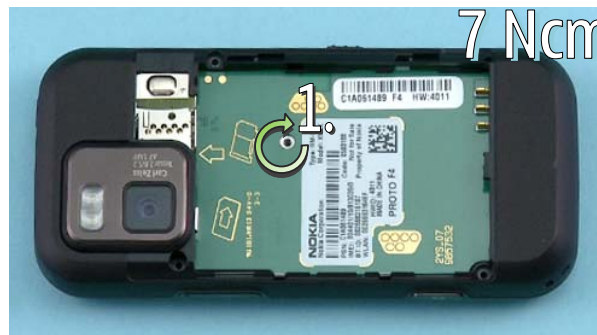
6) Tighten this M1.2X2, PANHEAD 2.5X0.6 T PLUS-4IPscrew to the torque of 7 Ncm.
