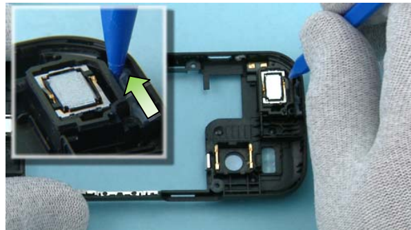
20) Release the GPS ANTENNA ASSEMBLY with the sharp end of the SS-93. Remove the antenna.
