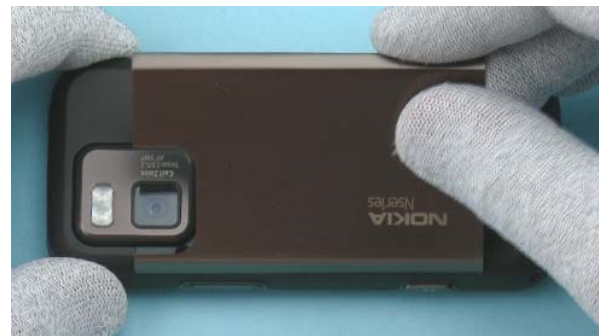
10) Make sure the battery cover is assembled correctly. First attach the hooks on the Camera/Volume key side. Then close the LOCK KEY side.
