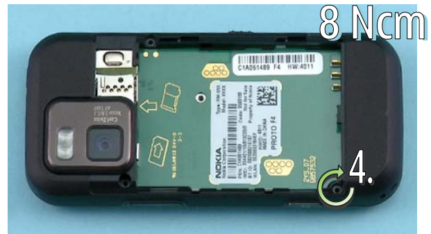
8) Tighten this M1.4x2.5 TORX PLUS-4IP screw to the torque of 8 Ncm.
