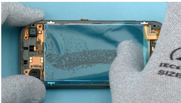
33) Protect the LCD with protective film.
