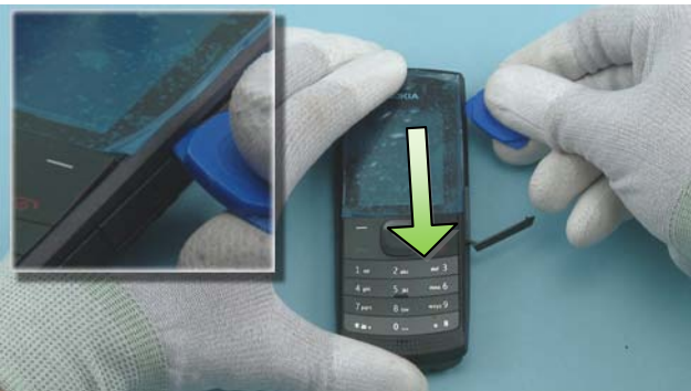
9) Release the sides of the A-COVER by sliding the SRT-6 to direction shown.
