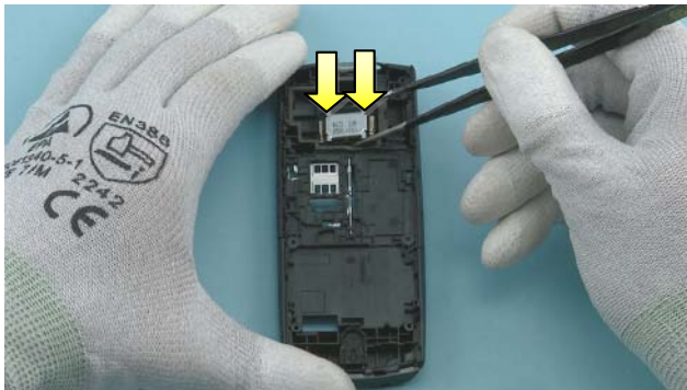
1) Insert the IHF SPEAKER with the tweezers. Make sure that the pins are correctly aligned.
