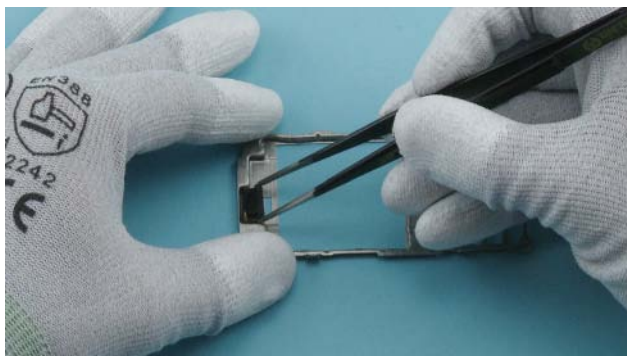
3) Place the EARPIECE to its place with the tweezers.
