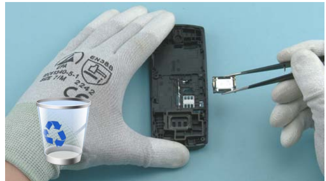
32) Remove it with the tweezers. Do not use it again. Discard it.
