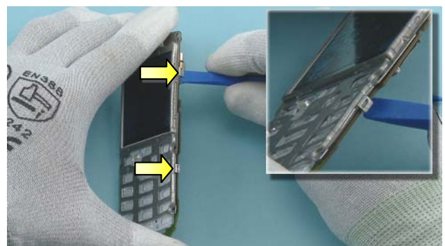
18) Release the two clips holding the UI SHIELDING with the SS-93.
