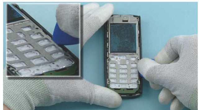
16) Use the SRT-6 to release the ENGINE BOARD.
