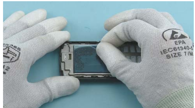
14) Protect the DISPLAY with a protective film.
