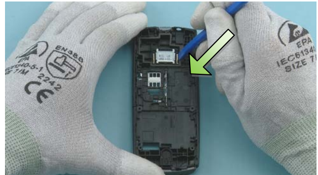
2) Push the IHF SPEAKER down from the shown place to activate the adhesive.
