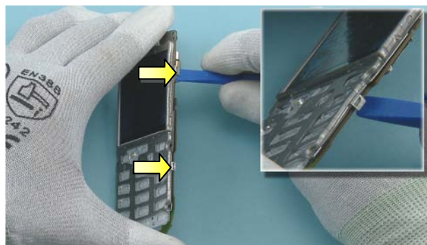
18) Release the two clips holding the UI SHIELDING with the SS-93.
