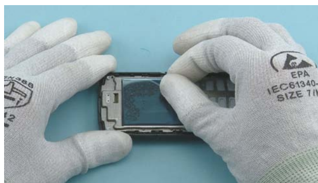
14) Protect the DISPLAY with a protective film.
