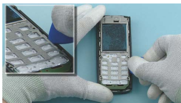
16) Use the SRT-6 to release the ENGINE BOARD.
