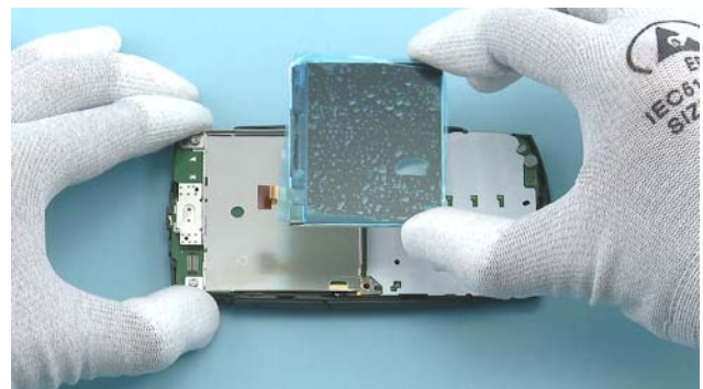
18) Lift up and remove the DISPLAY.
