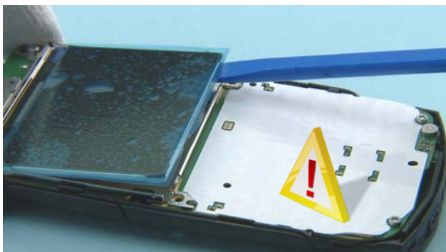
17) Detach also the other side of the DISPLAY. Be careful not to damage any nearby components.
