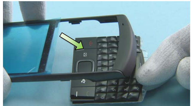
14) Pull the KEYMAT out as shown and remove it.
