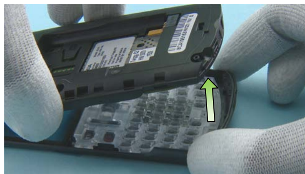
8) Lift up the D-COVER from the bottom side.
