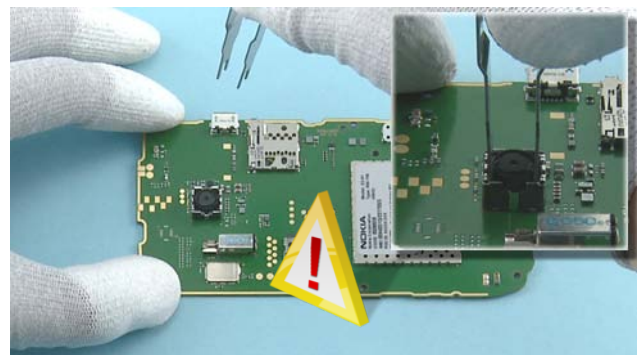
36) Remove the CAMERA with the SS-88 camera removal tool. Be careful not to damage any nearby components.
