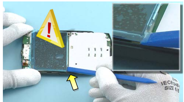
16) Use the SS-93 as shown to detach the DISPLAY. Be careful not to damage any nearby components.
