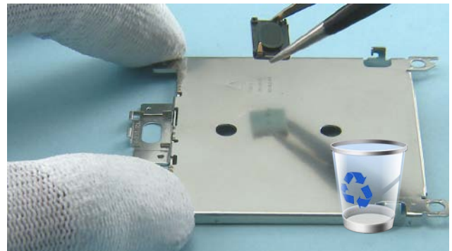
34) Use the tweezers to remove the EARPIECE. Do not use it again.
