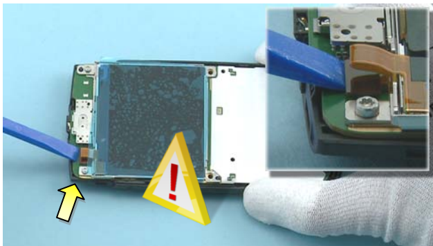
15) Use the SS-93 to carefully disconnect the DISPLAY connector.
