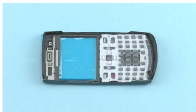
12) Protect the inside of the A-COVER with protective film.
