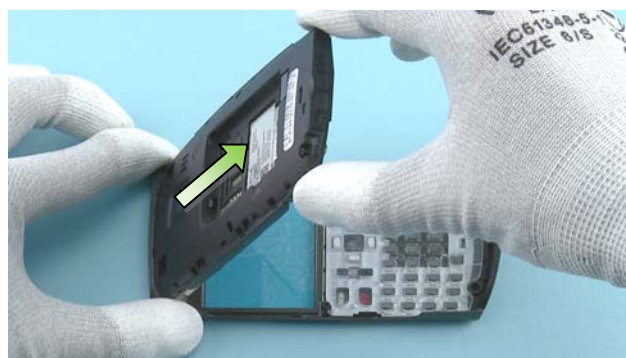
10) Remove the D-COVER as shown.
