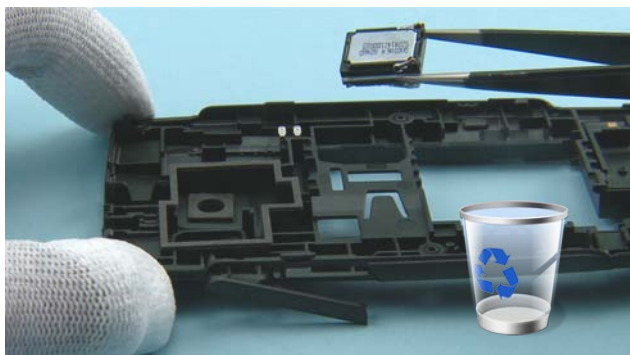
27) Use the tweezers to remove the IHF SPEAKER. Discard it.
