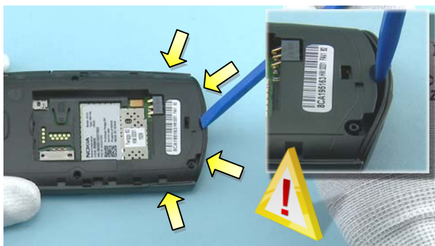
7) Insert the SS-93 between the A-COVER and the D-COVER. Use the SS-93 to detach all clips holding the covers together. Be careful not to damage the A-COVER.
