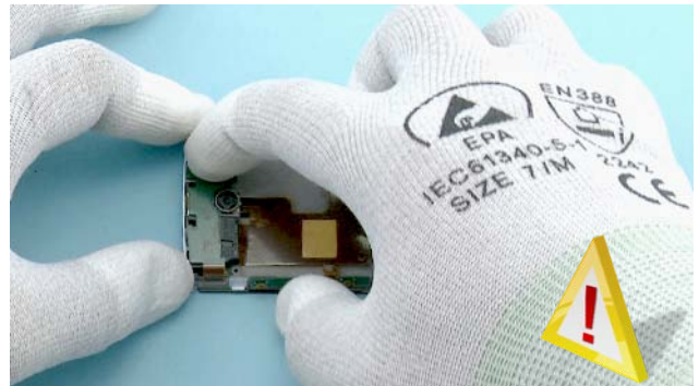
26) Turn the shown part of the ENGINE BOARD over and gently press it to lock up. Be careful not to damage any nearby components.
