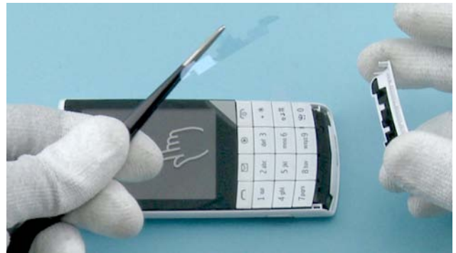
32) Remove the B-COVER DECO protective film with the tweezers.
