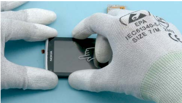
13) Lower down the bottom part of the TOUCH MODULE. Press gently from all sides of the TOUCH MODULE to activate the adhesive.
