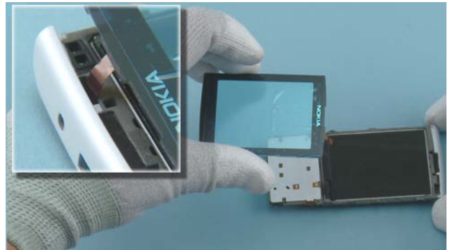
34) Pull the TOUCH MODULE connector through the opening and remove the TOUCH MODULE.
