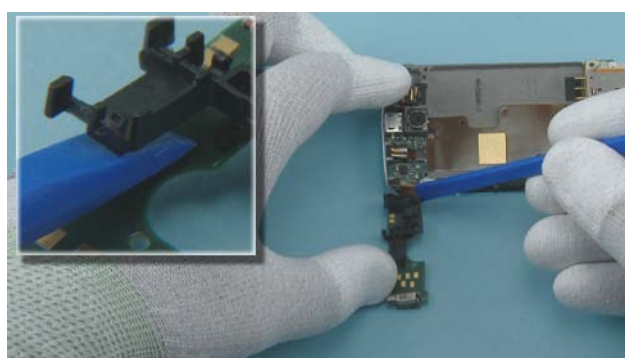
18) Use the SS-93 to release the MOUNTING ASSY.
