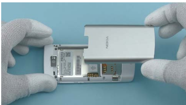
5) Lift up the BATTERY COVER. If there is a battery inserted remove it also.
