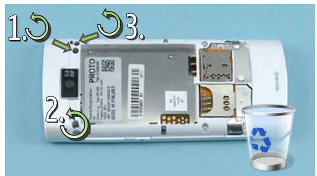
6) Unscrew the three TORX+ size 4 screws in the order shown. Do not use them again!
