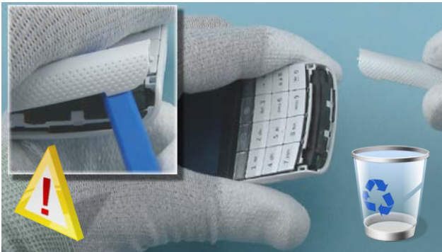
9) Remove the B-COVER DECO. Be careful not to damage the hooks holding the B-COVER. Do not use it again. Discard it.
