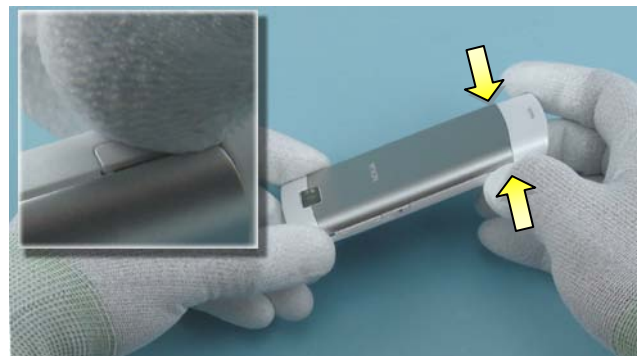
4) Push the BATTERY COVER release buttons on both sides.
