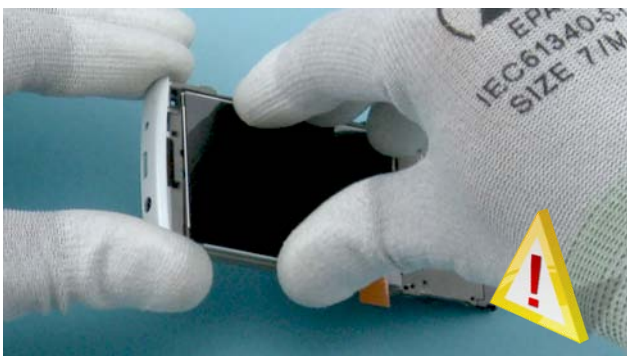
5) Press the sides of the LCD to activate the adhesive. Be careful not to damage the LCD.
