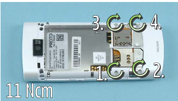
35) Tighten the four TORX + size 4 screws to the torque of 11 Ncm in the order shown.
