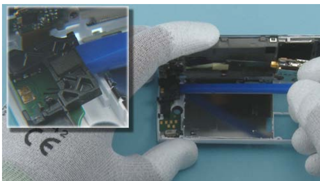
13) Carefully detach the top part of the ENGINE BOARD with the SS-93.
