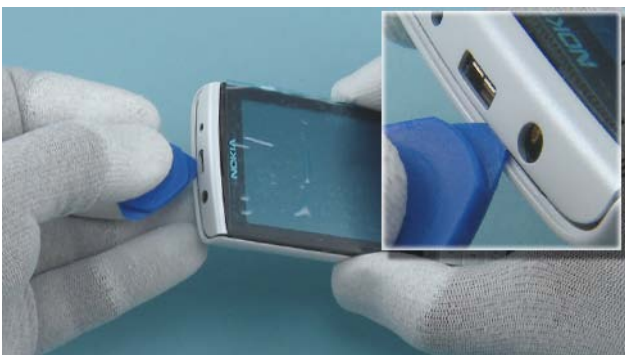
11) Release the top part of the A-COVER with the SRT-6.
