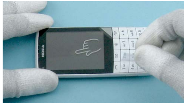
38) Remove the KEYMAT protective film.
