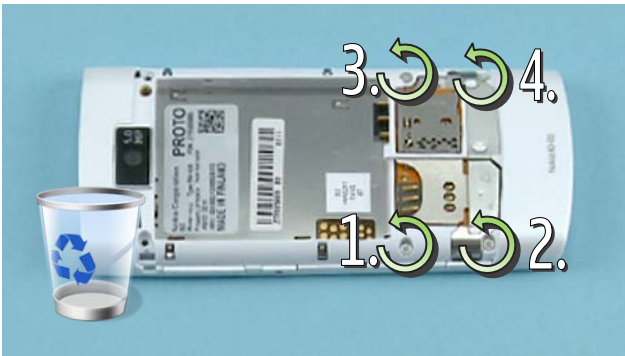
7) Unscrew the four TORX+ size 4 screws in the order shown. Do not use them again!
