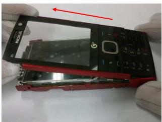
Push the A cover Assy to another side to release Remove A-COVER in arrow direction.
