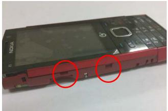
Unscrew the two 4IP torx plus screws.
