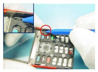
Take the A-COVER and release the first of the six clips with an SS-93.
