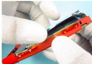
Use an SS-93 tool to lift up the LCD MODULE.
