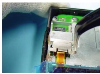
Then lift up LCD CONNECTOR SHIELDING with an angled tweezers on left-hand side
