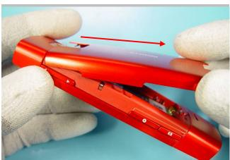
Release BATTERY COVER and remove it in arrow direction.
