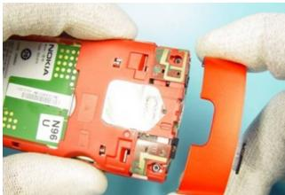
Remove the TOP COVER in arrow direction as shown.
