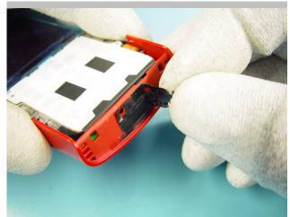
Remove the Bottom Deco in arrow direction.
