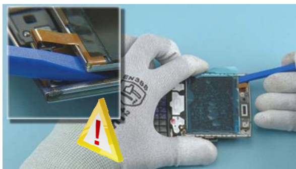
17) Use the SS-93 to lift up the LCD. . Be careful not to damage the connector!
