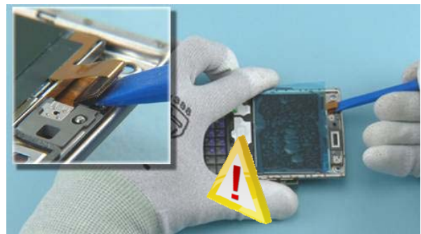
16) Use the SS-93 to open the LCD connector. When opening the connector, be careful not to damage the connector or any nearby components.
