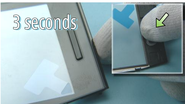
41) Check that the MENU / HOME KEY is aligned correctly in to the A-COVER TOUCH ASSEMBLY. The MENU / HOME KEY should be located on the center. Press the MENU / HOME KEY for 3 seconds to activate the adhesive.
