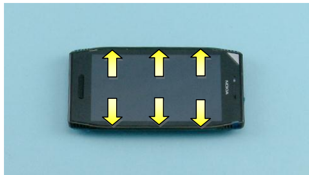
56) Check the shown gaps for defects in installation. Please refer to the gap specification document for accurate values.
