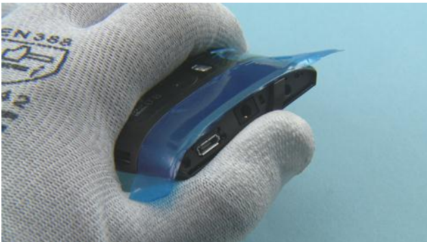
51) Test that the device can be powered up properly. If the device does not power up, this may be caused by the Dipro LED short circuit. In this case please follow the instructions how to reset a short-circuited Nokia X7-00 on page 47.
