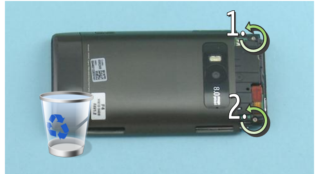
13) Unscrew the two Torx+ size 4 screws in the order shown. Do not use them again. Discard them.
