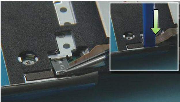
33) Use the tweezers to place the DISPLAY CONNECTOR RETENTION CLIP as shown. Press the DISPLAY CONNECTOR RETENTION CLIP with the SS-93 to fasten it correctly.
