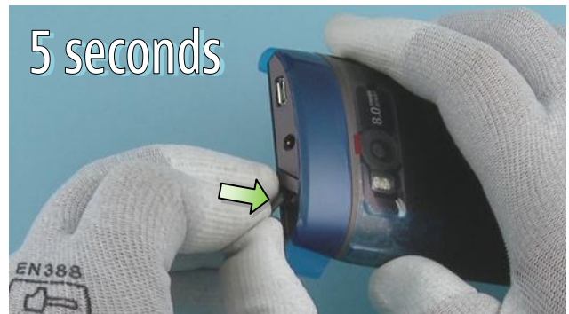
70) Place the LOCK KEY FACE PLATE to the TOP END CAP and press it gently for 5 seconds to activate the adhesive.
