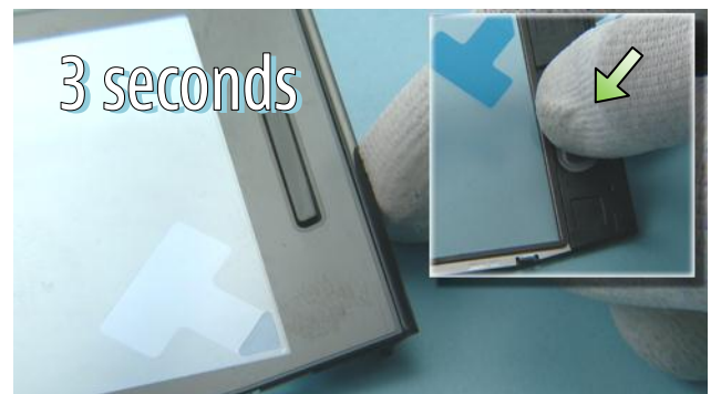
46) Check that the MENU / HOME KEY is aligned correctly in to the A-COVER TOUCH ASSEMBLY. The MENU / HOME KEY should be located on the center. Press the MENU / HOME KEY for 3 seconds to activate the adhesive.
