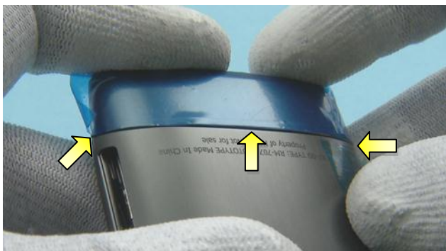
55) Check the shown gaps for defects in installation. Please refer to the gap specification document for accurate values.
