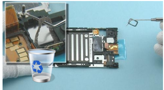
51) Remove the EARPIECE ADHESIVE with dental tool. Do not use it again. Discard it.
