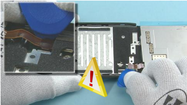
30) Open the DISPLAY connector with the SRT-6 as shown. Be careful not to damage the DISPLAY connector.
