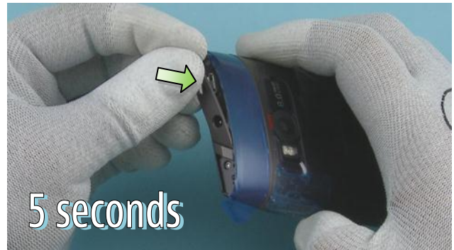
68) Place the AV FACE PLATE to the TOP END CAP and press it gently for 5 seconds to activate the adhesive.
