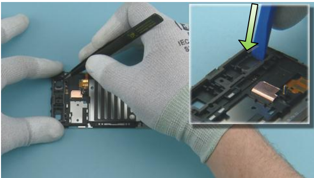
9) Place the first IHF SPEAKER MESH with the tweezers. Press it gently with the SS-93 to activate the adhesive.
