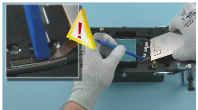
36) Use the SS-93 to connect the DISPLAY CONNECTOR. Be careful not to damage the connector.
