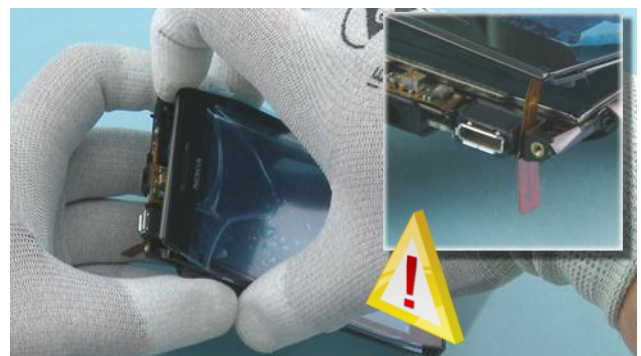
17) Lift slightly up the top end of the A-COVER TOUCH ASSEMBLY. Be careful not to damage the TOUCH FLEX connector.
