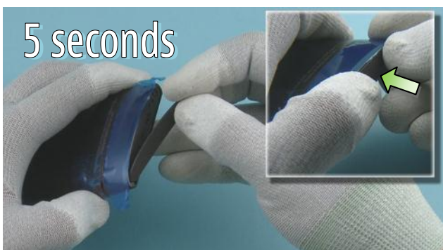
59) Place the BOTTOM END FACE PLATE to the BOTTOM END CAP and press it gently for 5 seconds to activate the adhesive.
