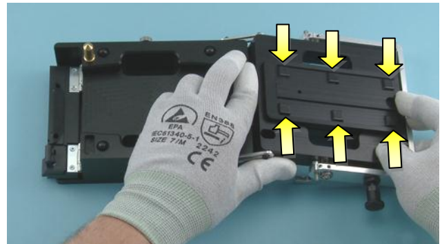
58) Turn over the press plate so that rubber bumps are on top.
