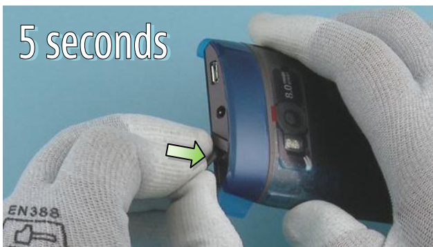
63) Place the LOCK KEY FACE PLATE to the TOP END CAP and press it gently for 5 seconds to activate the adhesive.
