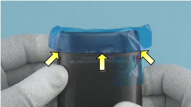
31) Check the shown gaps for defects in installation. Please refer to the gap specification document for accurate values.
