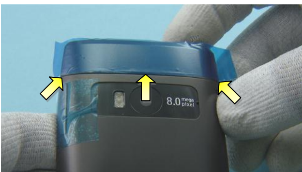
53) Check the shown gaps for defects in installation. Please refer to the gap specification document for accurate values.
