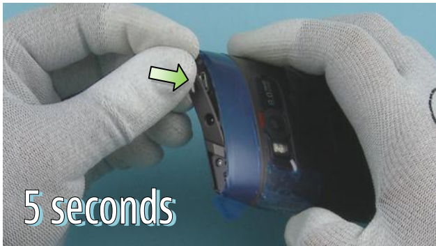
61) Place the AV FACE PLATE to the TOP END CAP and press it gently for 5 seconds to activate the adhesive.
