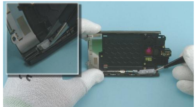
16) Use the tweezers to place the CAMERA KEY and the VOLUME KEY.
