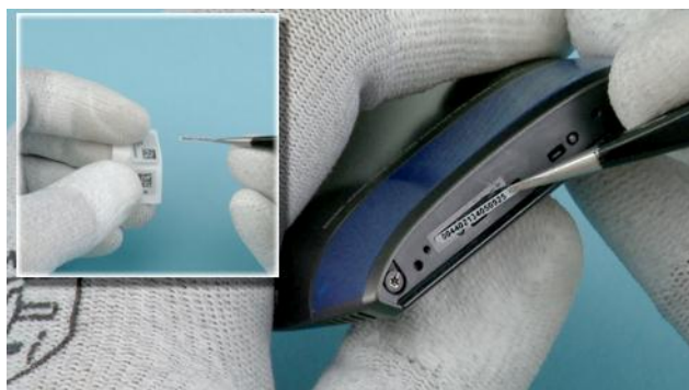
57) Note that this step is for Level 3 only! Take the second TYPE LABEL and attach it to the BOTTOM END CAP in the shown place.
