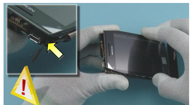
48) Guide the TOUCH FLEX to its gap as shown. Be careful not to damage the flex! Start placing the A-COVER TOUCH ASSEMBLY to its place from the shown side. Note that the A-COVER TOUCH ASSEMBLY has to be assembled in a slight angle.
