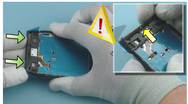
28) Place the BOTTOM END CAP, by first sliding it in partially. Push it from the back side to lock the shown clip into its place. Be careful not to damage the clip. Press the BOTTOM END CAP to its place by pressing from the shown sides, and from the back of it.
