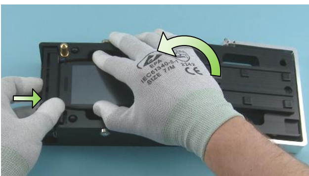
59) Place the device in the jig as shown and lock the bottom end of the jig. Then close the top part of the jig and lock it.
