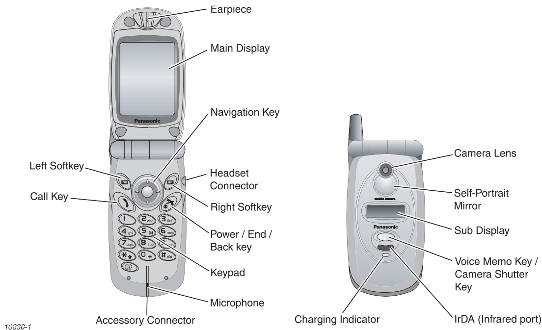
Figure 3.1: Location of Controls and Indicators
