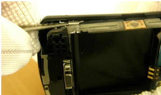
**10**1) Assemble the volume key pad with front.
