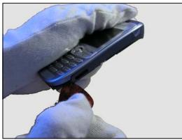
and release the *front cover* by sliding the guitar pick from bottom to top along each side of the phone.
