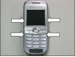
Tighten four **new** screws with 11 Ncm torque using torx bit no. 6 in order 1-4, as indicated in the adjacent picture.
