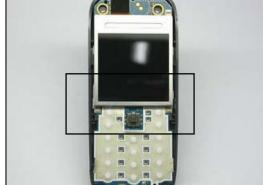
Place the PCB inside the frame.
