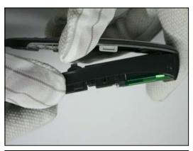
Use your fingers to press on each side of the *front cover* as indicated by the arrows, to make it securely snapped.
