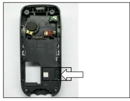
Push and remove the *IrDA window* from the outside of the frame.
