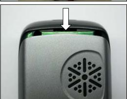
Remove the battery cover by lifting it up.
