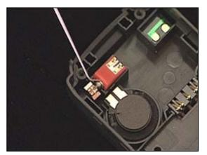
Use the tweezers to place the *vibrator* in its proper position and press gently, without touching the contacts, until it reaches the bottom of the cavity.
