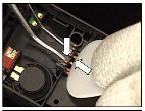
until the *battery connector* drops down into its proper position.
