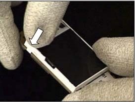
Press at these four corner spots to make the LCD attached to the adhesive on the PBA.
