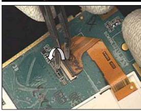
and pull the flex cable out of the ZIF connector by using the flex film assembly tool.
