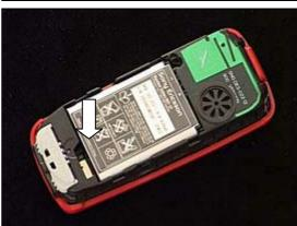
Position the *rear cover* into the frame cabinet at the bottom and put the two parts together.
