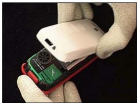
Press on both sides at the top until the *rear cover* is securely snapped to the frame cabinet.
