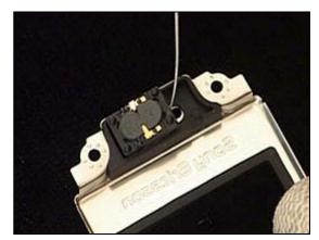
Use the tweezers to place the *earphone* in its proper position and press gently, without touching the contacts, until it reaches the bottom of the cavity.
