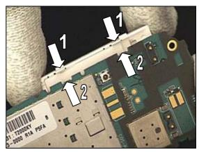
Press on the top left corner of the LCD to snap the third hook onto the PBA.
