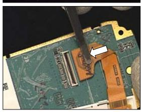
Secure the connection by turning and pressing the black clamp.
