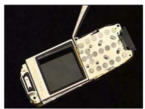
Place the light guide on the lower part of the metal carrier.
