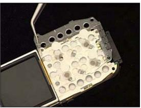
Tighten five **new** T6 screws in the order 1 - 5 by using 11 Ncm torque.
