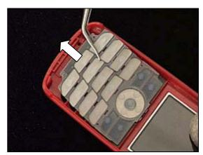
Place the *keypad* inside the front cover and press with your fingers to attach it to the front cover.
