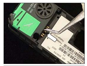
until the battery connector falls out of the frame cabinet.
