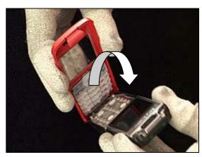
Press the *front cover* against the frame cabinet so that both sides and the top of the *front cover* are securely snapped to the frame cabinet.
