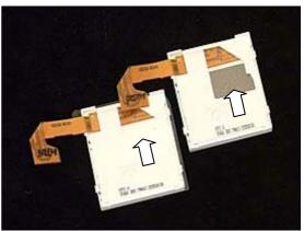
Check that the black ZIF connector clamp still is open and then insert the flex film into the connector.
