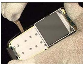
Press on the *PBA* through the opening of the frame cabinet (1) and simultaneously release the *PBA* with the front opening tool (2).
