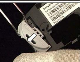
Put the *strap holder* in position and push it onto the frame cabinet ...
