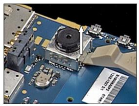
Position the camera tool into the camera socket, as shown in the picture.
