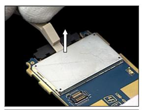
Loosen the *BB Shielding Cover* on the other side using the Front Opening tool shown in the picture.
