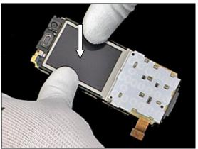
Press down and secure snap hooks at bottom end of *PCBA*.
