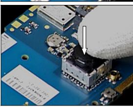
Position the 2.0 Pixel Camera Shield into the place as shown in the picture using fingers.
