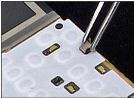
Add the *Function Key Conductive Gasket* into position as shown in the picture using the tweezers.
