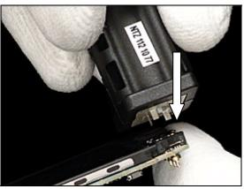
Loosen the camera from socket by lifting tool upwards.
