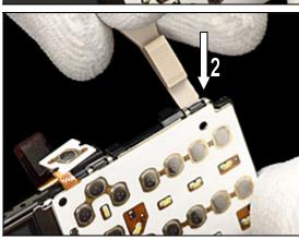
Lift off the Key foil Dome Assy as shown in picture.
