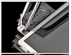
Secure the receiver conductive gasket using tweezers.
