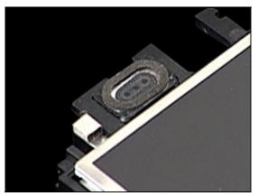
Remove the receiver conductive gasket using tweezers.
