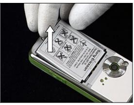
Grip Battery as shown in picture and lift out from phone.
