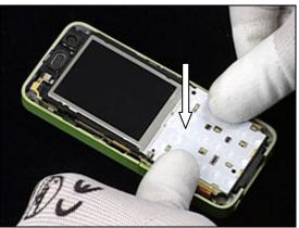
Press down on *PCBA Assy* to secure into the *Main Frame Assembly* at the top end of phone second.
