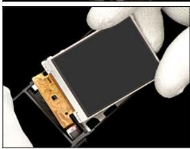
Check placement of LCD and flex location pin is positioned correctly.
