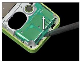
Grip Antenna Assy and lift away from Main Frame Assembly.
