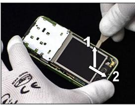
Grip at top of *PCBA Assy* and lift to remove it from *Main Frame Assembly* as shown in picture.
