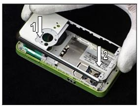
Press down the bottom end of phone to secure snap hooks as shown in picture.
