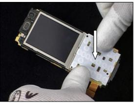
Secure Keyfoil Dome Assy connector using finger.
