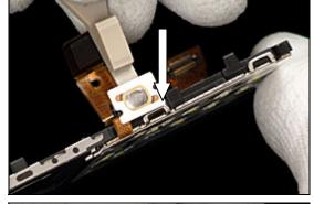
Loosen 1<sup>st</sup> snap hooks using side opening tool.
