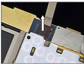
Grip LCD Frame Assy with fingers and lift from PCBA.
