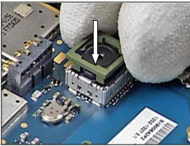
Press down on the camera tool with two fingers, until camera tool completely enters the camera socket as shown in picture.
