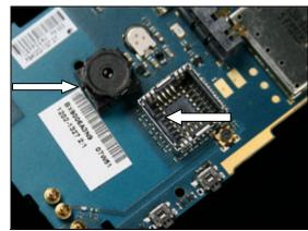
Position the *Camera 2Mega Pixel* into place as shown in the picture using fingers
