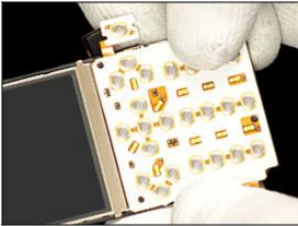
Use Tweezers to secure the positioning of camera button.
