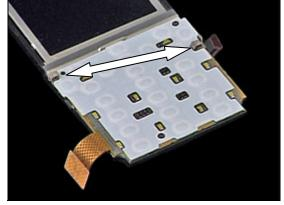
Add the *Function Key Conductive Gasket* into position as shown in the picture usin*g* the tweezers.
