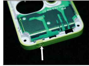
Remove On/Off Key using tweezers.
