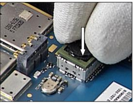
Remove the Camera 2Mega Pixel using fingers and lift out of the Camera Socket.
