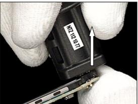
Remove QCIF VGA Camera by using tweezers.
