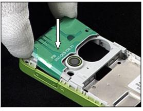
Position Antenna Assy into correct position using fingers.
