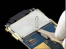
Remove the *BB Shielding Cover* using fingers as shown in the picture.
