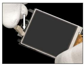
grip at top of LCD and lift out of LCD Frame
