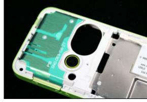
Push the *Camera lens Assembly* using the Nylon Pointer shown in the picture.
