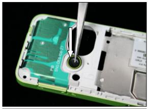
Secure the *Camera lens Assembly* using finger, and check the positioning and alignment.
