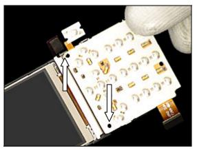
Press down and secure the Key Foil Assy.
