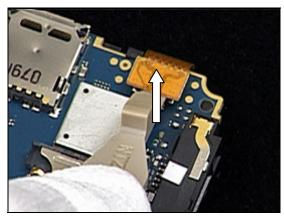
Use side opening tool to unlatch all 5 snap hooks as shown in picture by the arrows.
