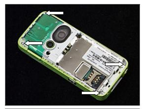
Insert guitar pick tool as shown in picture and unlatch snap hooks along the side of the phone as shown by the arrow.
