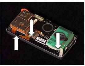
Once all Front Cover snap hooks have been released, remove the front cover.
