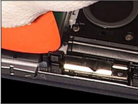
BE CAREFUL NOT TO DAMAGE OR SCRATCH THE PLASTICS AND THE CAMERA SWITCH!
