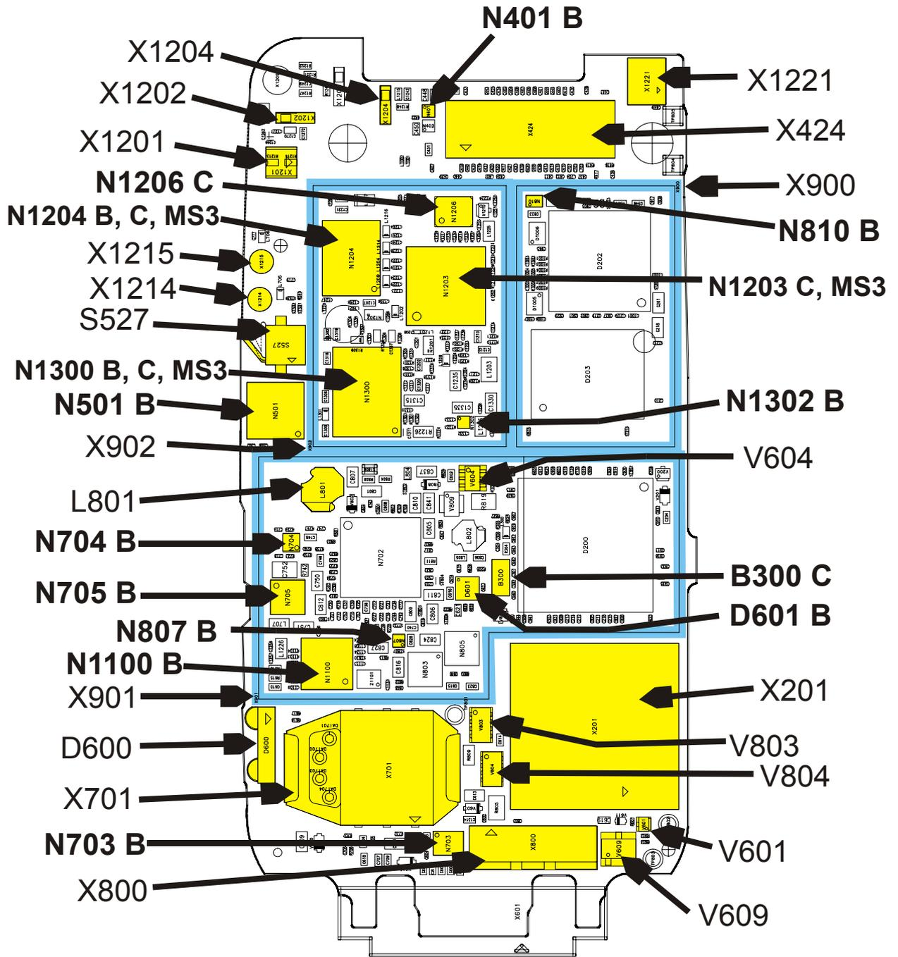
B - BGA Rework Equipment Required
