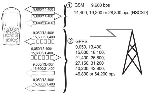
Figure 4 A comparison between GSM and GPRS
