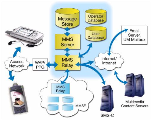
Figure 3. The architecture of MMS
